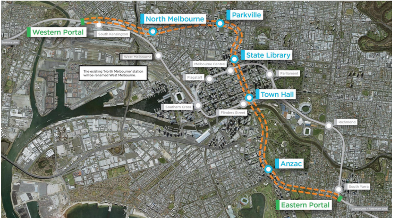
The proposed Metro Tunnel Project showing the location of the five stations between the Eastern and Western Portals.
