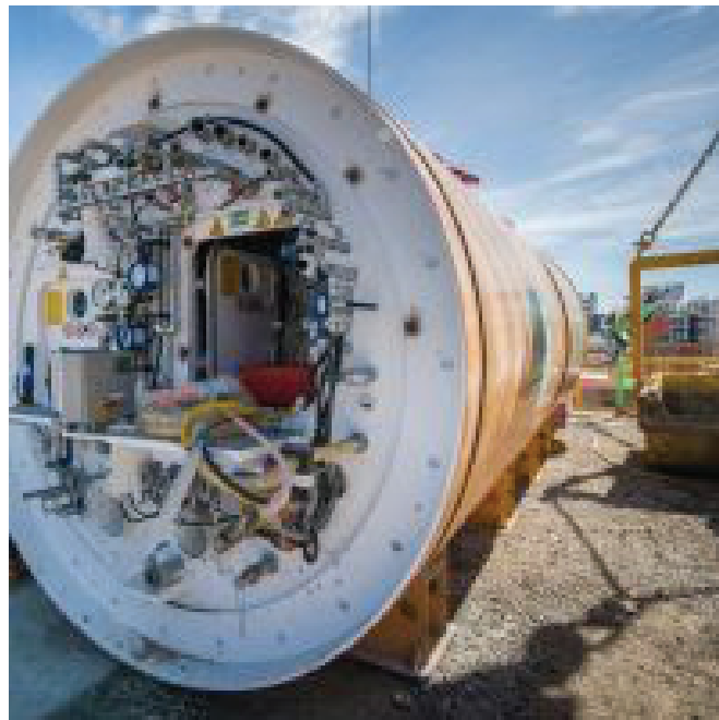
Widening work on the West Gate Freeway and a mini Tunnel Boring Machine (TBM) which will be used to divert the North Yarra Main Sewer.
