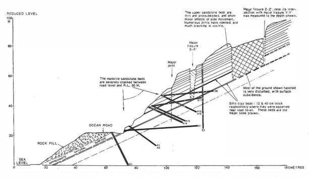
Figure 8—Section VII of Windy Point landslide area showing the sliding rock mass, the inclined bedding planes and the several types of bores drilled. As indicated, the bores showed the location of the crush zones, cavities and the more solid rock under the slide planes.
