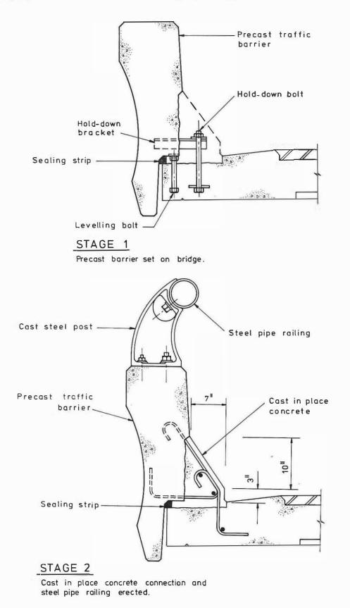
Figure 4-Precast concrete traffic barrier used on the West Footscray Bridge, Princes Highway West.
