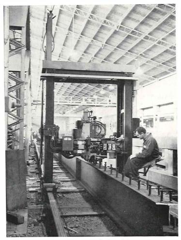
Plate 9—Production friction welding machine
