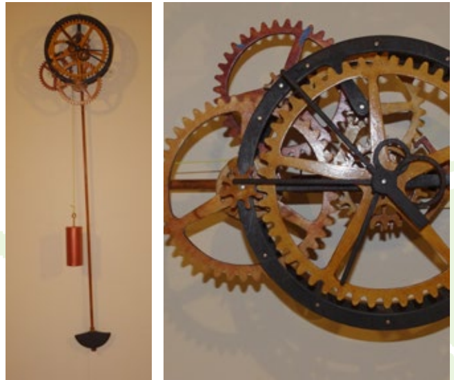
These pictures show the gears for the clock (top), and the finished clock (bottom left). The finished gears in Baltic Birch plywood (bottom right).
