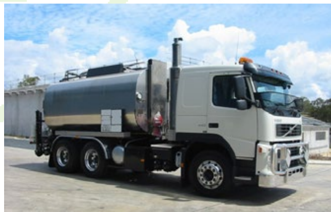
A modern Volvo 12,000 L Bitumen Sprayer
