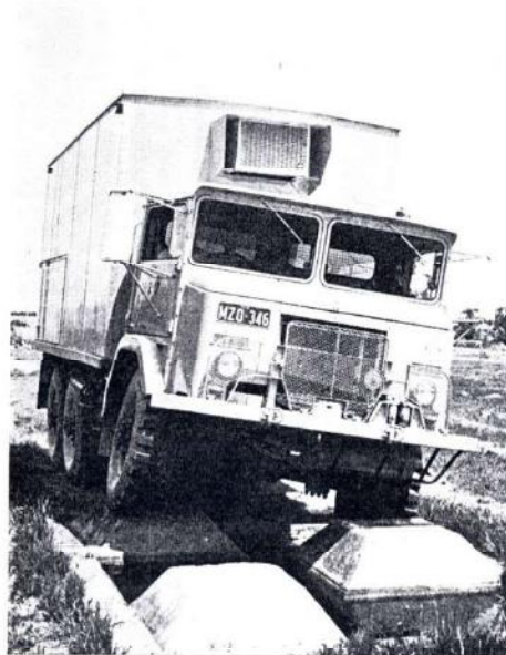
Plate 8—Penetrometer Testing Vehicle during trials at the Army's Monegeeta proving ground.
