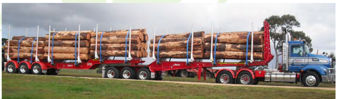
This is a properly loaded B-Double. The load is secured and higher in the middle.
