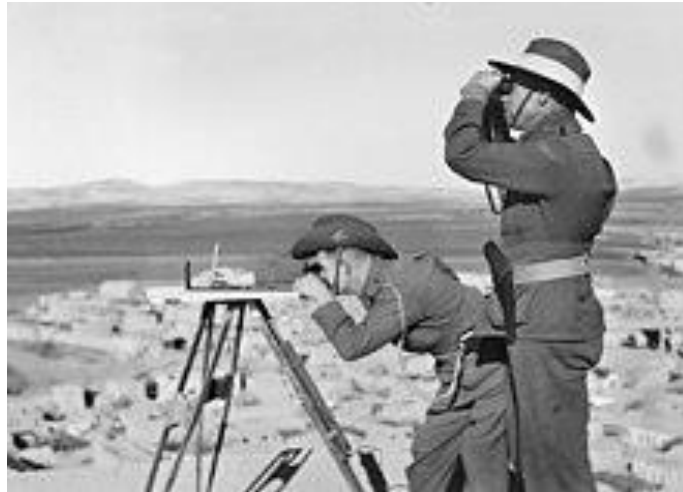
Soldiers from the Australian 2/1st Corps Field Survey Company, near the Turkish–Syrian border, December 1941, mapping the topography using a plane-table.
