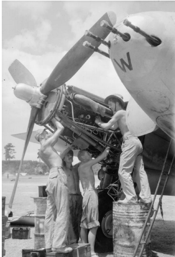
Ground crew of No. 110 Squadron RAF service the starboard engine of a de Havilland Mosquito FB Mark VI at Joari, India.
