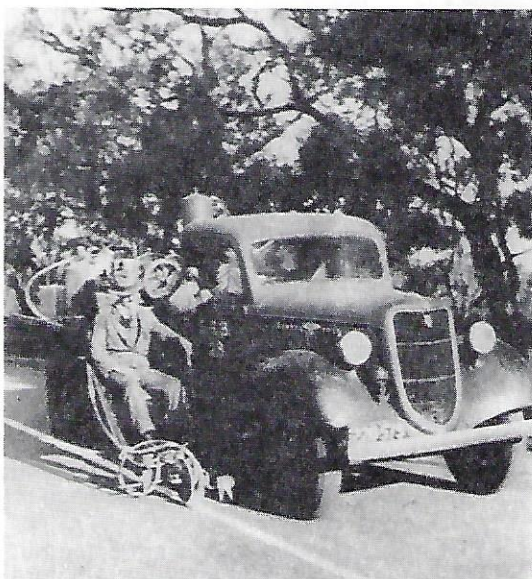
Linemarking began in the early 1930s when a number of hazardous curves were marked with a solid centreline. In 1936 the CRB bought its first linemarking machine for £ 136 — it was a two horse power motor driving a
