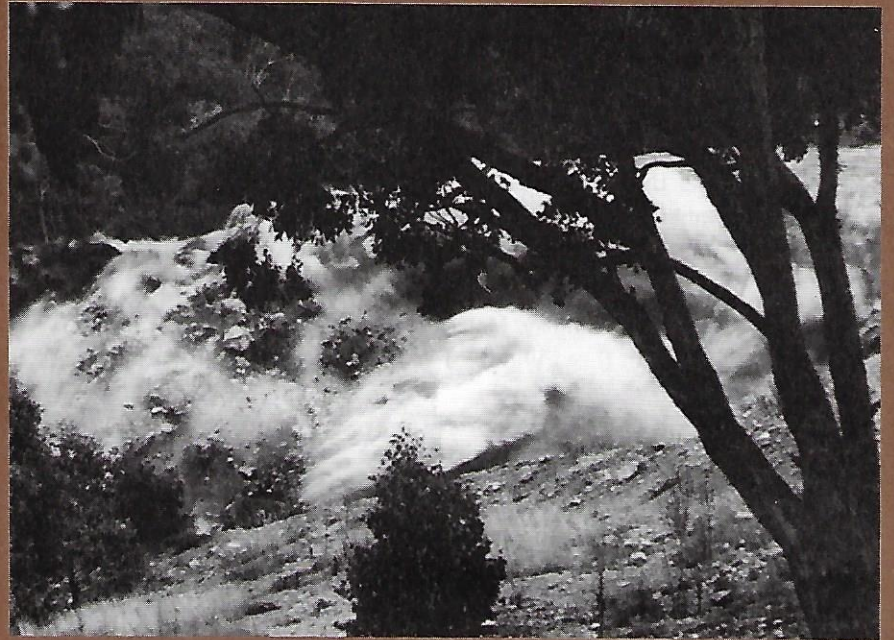
Above and below: Starting the day off with a bang. Blasting for material at the quarry. The material is being used for sub-base on the Western Freeway bypass of Melton.
