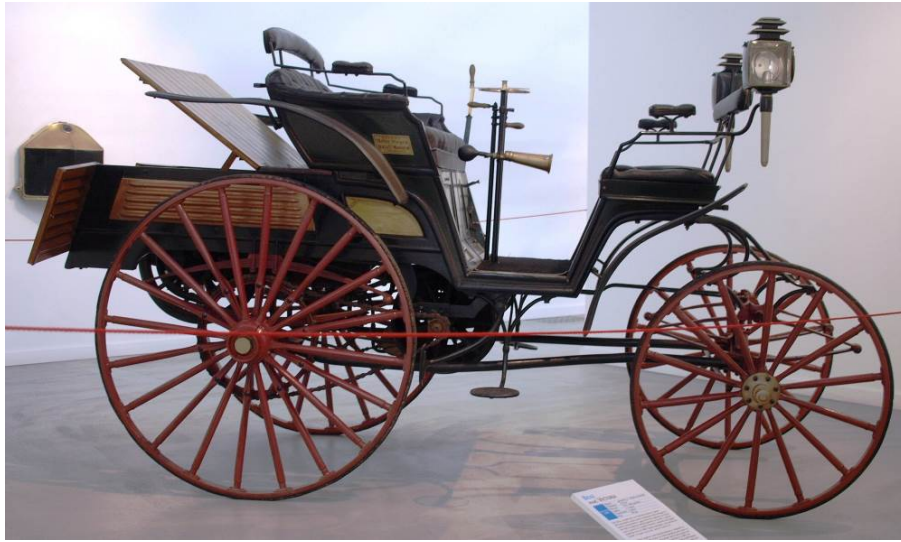
The Benz Victoria. It had tiller steering and its single cylinder 3 kW engine drove the car via a belt clutch at speeds of up to 20 km/h. Photo: Medak at Turin via Wikipedia Commons.
