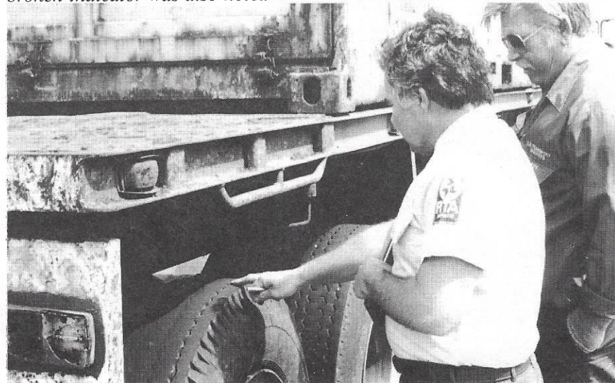
Rob pointing out an unacceptable tyre tread - the broken indicator was also noted
