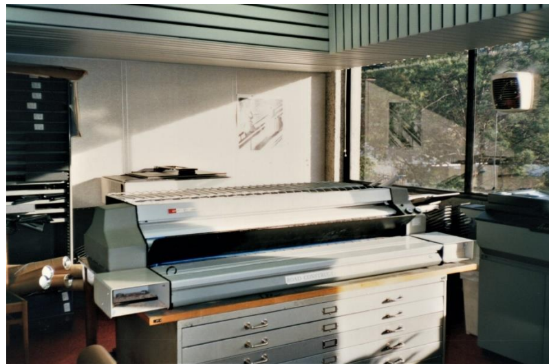
1985 – Print room at Bridge division. Includes dyeline printer for all the plans.
