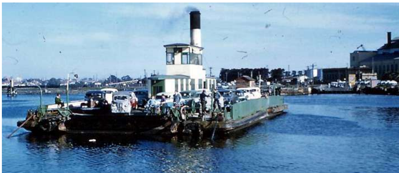
Figure 4.1b Steam-powered cable ferry (the two cables can be seen at the rear of the ferry) crossing the Yarra towards the right bank. Newport Power station is partly visible on the right side of the scene. The Author
