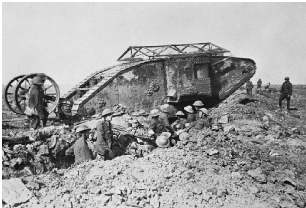
British Mark I tank with anti-bomb roof and "tail," 1916.
