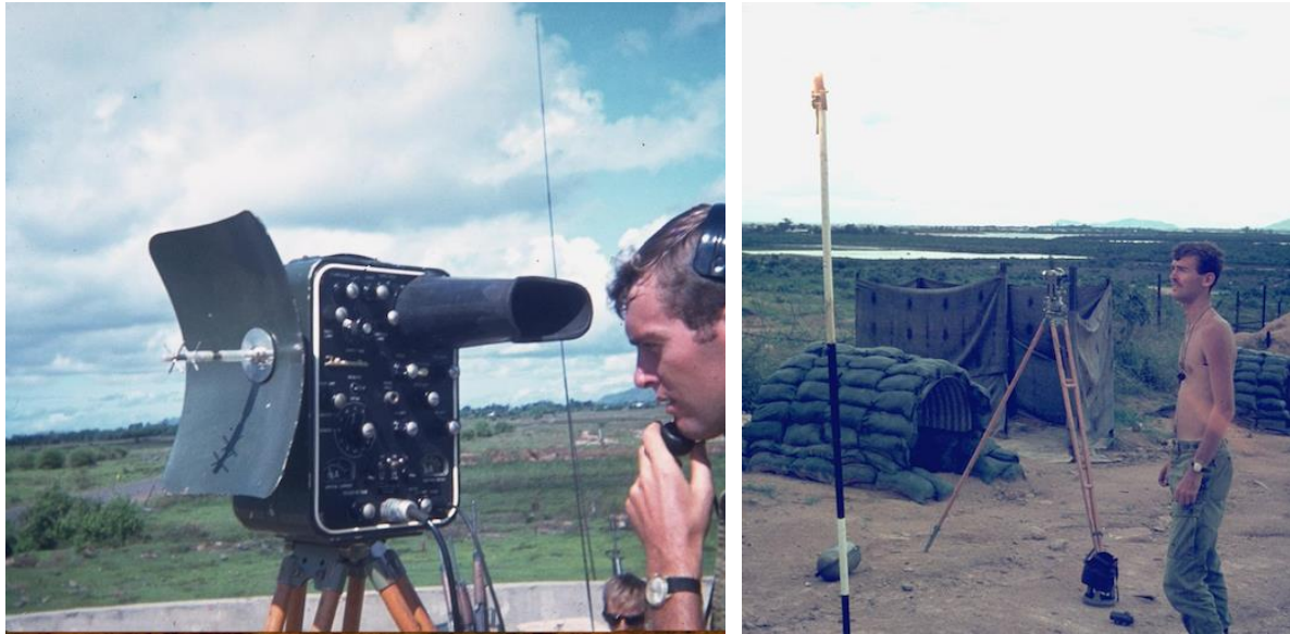
Mike using a tellurometer (left) and the Wild 2 theodolite (right).
