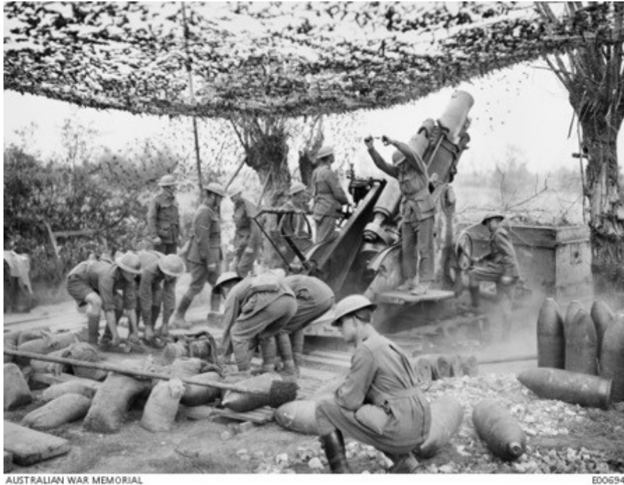
A 9.2 inch Howitzer of the 36th Heavy Artillery Group in action near Ypres in September 1917 – a month before Frederick arrived. The Gunner with his hands above his head has just pulled the lanyard that fires the vent tube which ignites the bag charge propelling the shell – much like a naval gun. This photograph was taken by the renowned war photographer, Frank Hurley.
