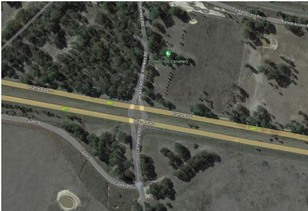
An aerial view of the intersection of the Hume Highway and Wenkes Road showing the wide median treatment. The fatal crash occurred at the upper right yellow dot. Melbourne is to the right and Wodonga to the left.
