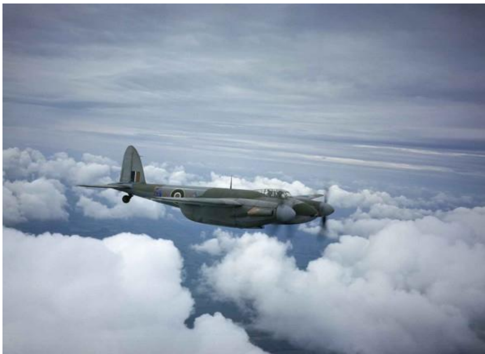
A De Havilland Mosquito of No 456 Squadron, flying from Middle Wallop, in flight. The wartime Censor has scratched out the wing-tip antennae of the Airborne-Interceptor radar.
