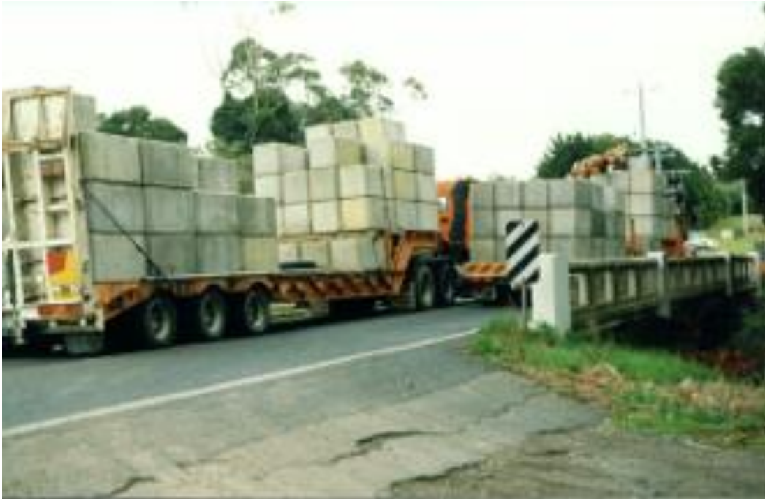
Load Testing In-service Bridge with Twin 100t semi-trailers
