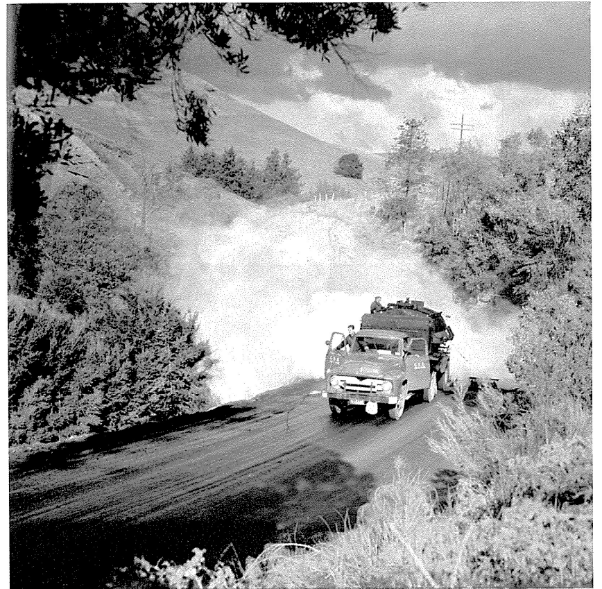
Modern 800-gallon sprayer in operation, 1962.
