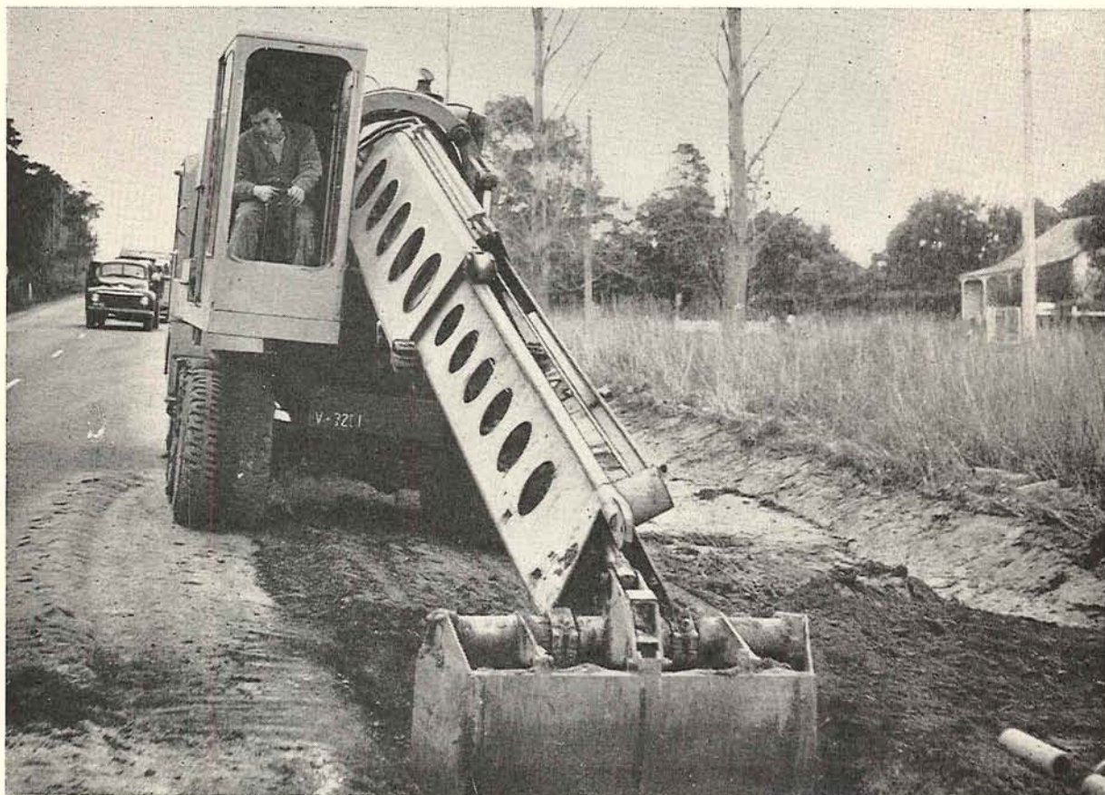
Plate 1.—“ Gradall ” combined excavator, back-actor, ripper, and grader.
