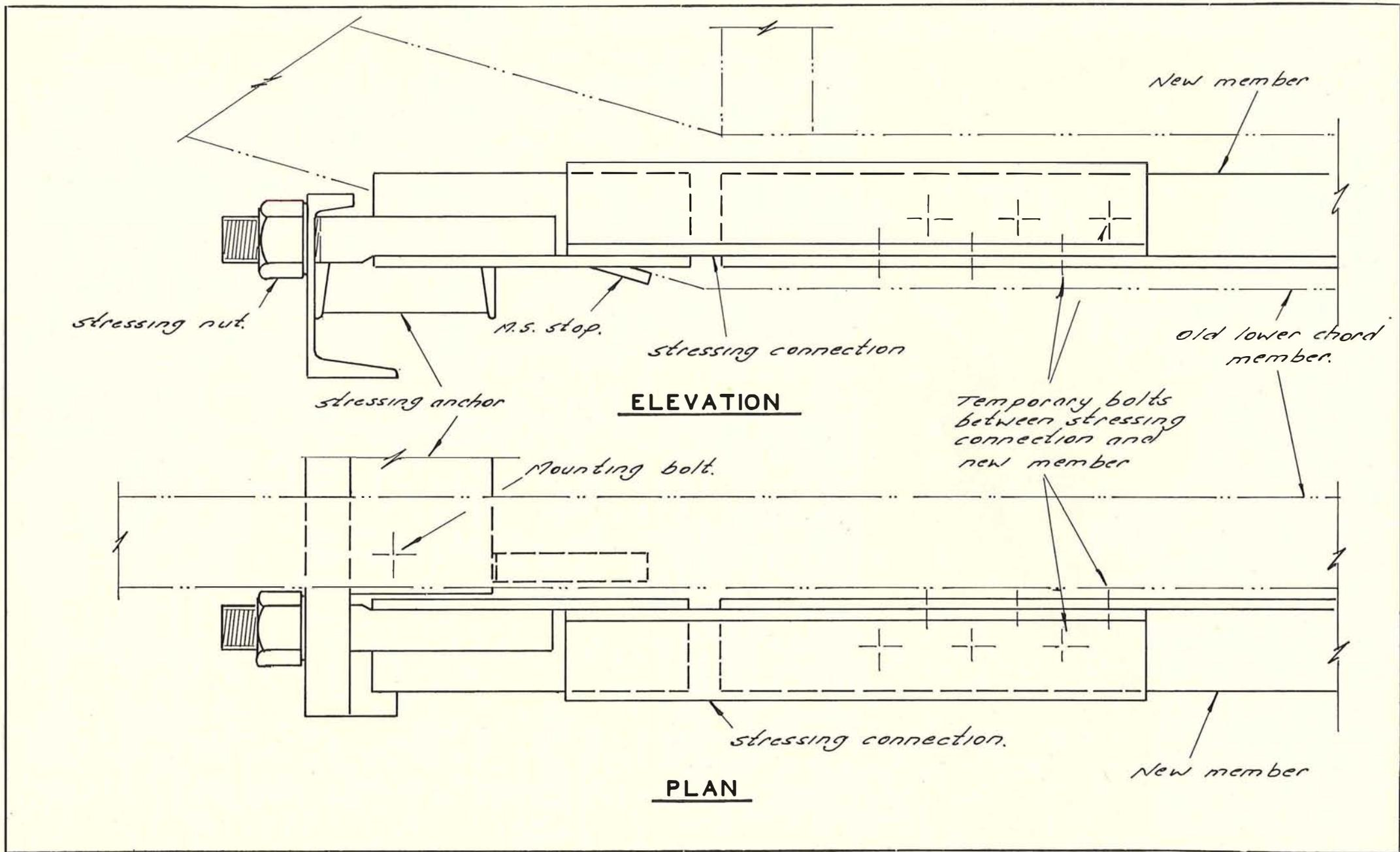
Figure 4.—Arrangement for prestressing new strengthening member at Bemm River Bridge.
