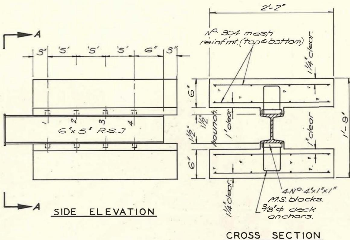
Figure 3.—Test specimen for shear connector tests.
