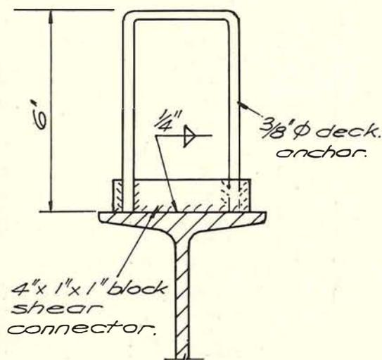
Figure 2.—Shear connector used in bridge construction.
