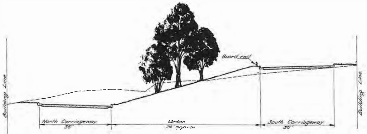
Proposed treatment—Trees on a wide median protected by a guard rail.
