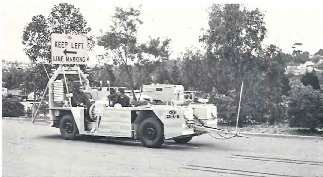
Line Marking — New machine designed and constructed at the Central Depot, Syndal.
