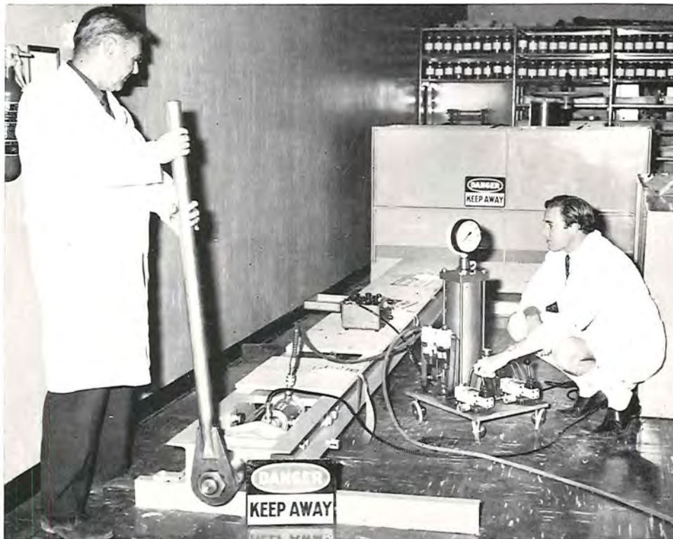
Plate 4—Equipment for the Measurement of Relaxation of Stress in Reinforcing Tendons.
