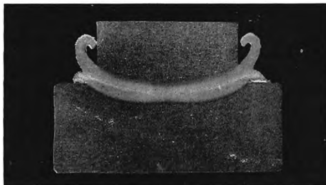
Plate 12—Cross section of a \frac{3}{4} in. friction welded stud, x 2.
