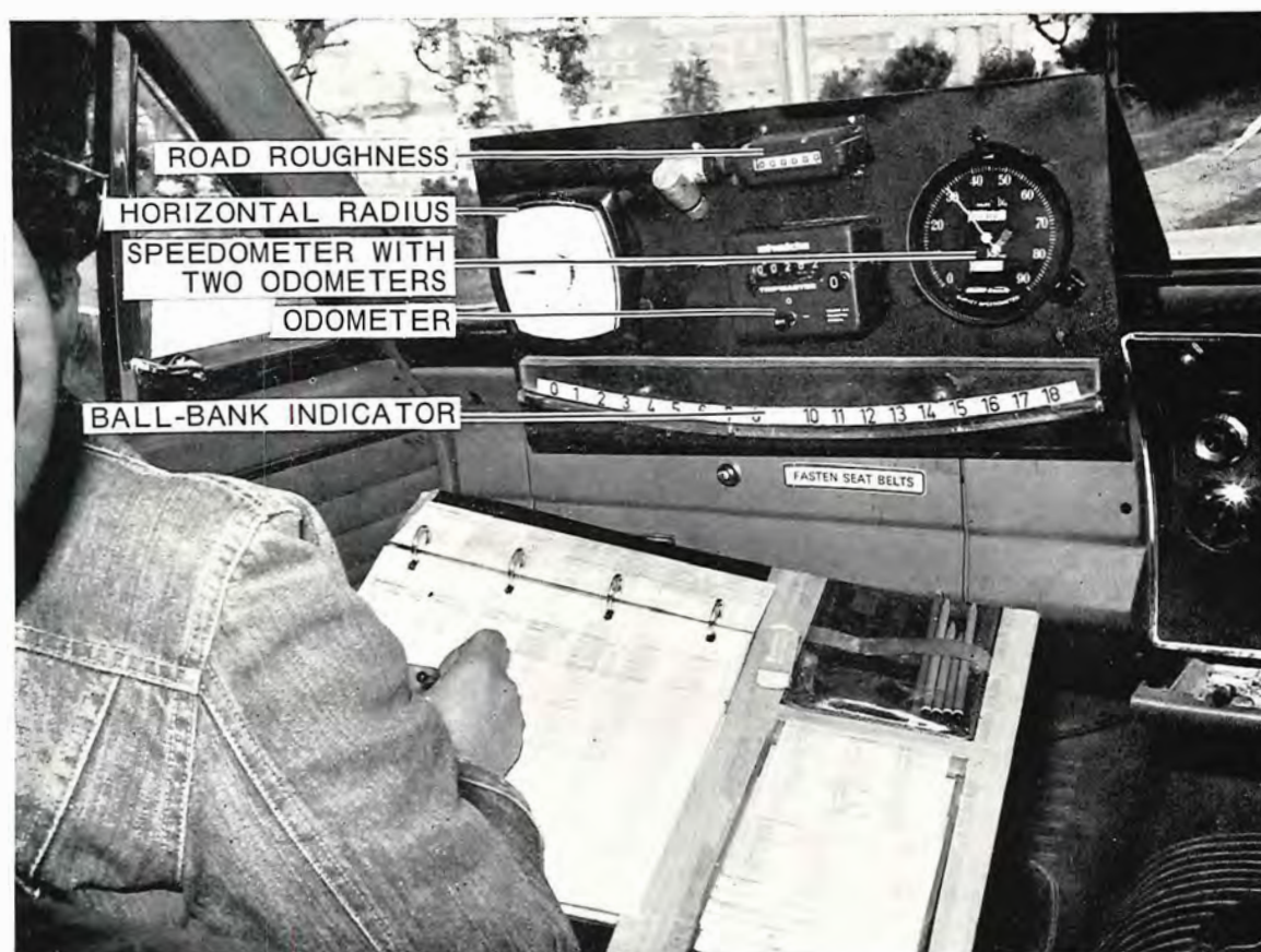
Plate 6—Road inventory vehicle—instrument panel and recording position.
