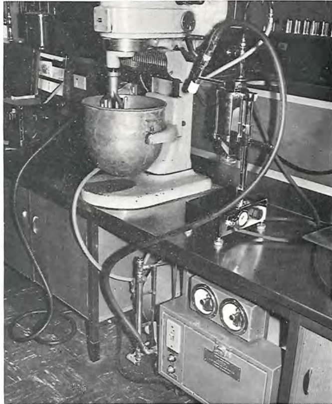
Plate 17—Laboratory apparatus for production of foamed bitumen for testing purposes. A measured quantity of bitumen is held in the cylinder at the top right of the photograph. Compressed air is used to force the bitumen up into the nozzle to the left of the cylinder. Steam from the generator below the bench passes through the same nozzle and causes the bitumen to foam or expand. The foamed bitumen is mixed with soil in the bowl beneath the mixer.
