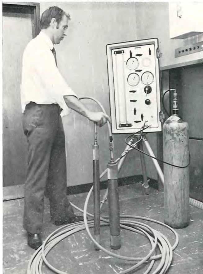
Plate 10—Menard Pressuremeter assembled, showing volumeter, gas supply to apply pressure to the water, probes and connecting conduit.
