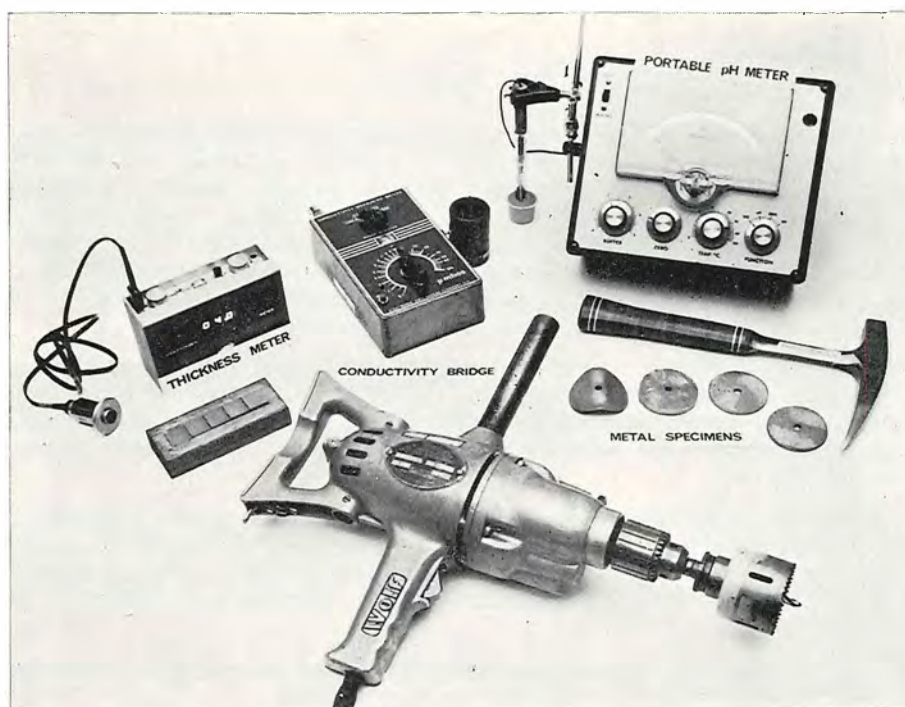
Plate 11—Portable equipment used in tests of corrosion of galvanized metal culverts, and some sample metal specimens obtained.
