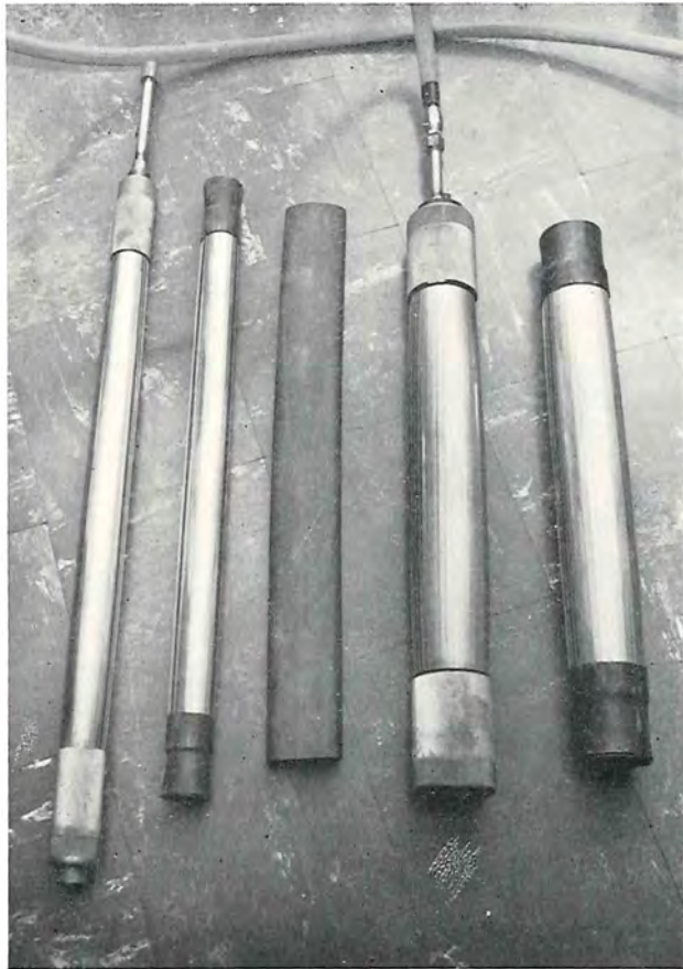
Plate 9—Menard Pressuremeter. Probes with spare metal sheaths and rubber membrane. From left to right, small probe, metal sheath, rubber membrane, large probe, metal sheath. The metal sheaths are used for rock testing and the rubber membranes for soil testing.
