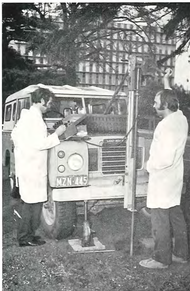
Plate 10—Penetrometer in operation.
