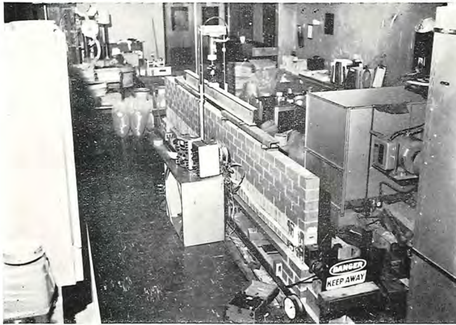
Plate 15—Prestressed Brick Lintel under Test.
