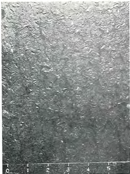
Plate 17 Surface BEFORE "coking" (Note surplus bitumen on surface)
