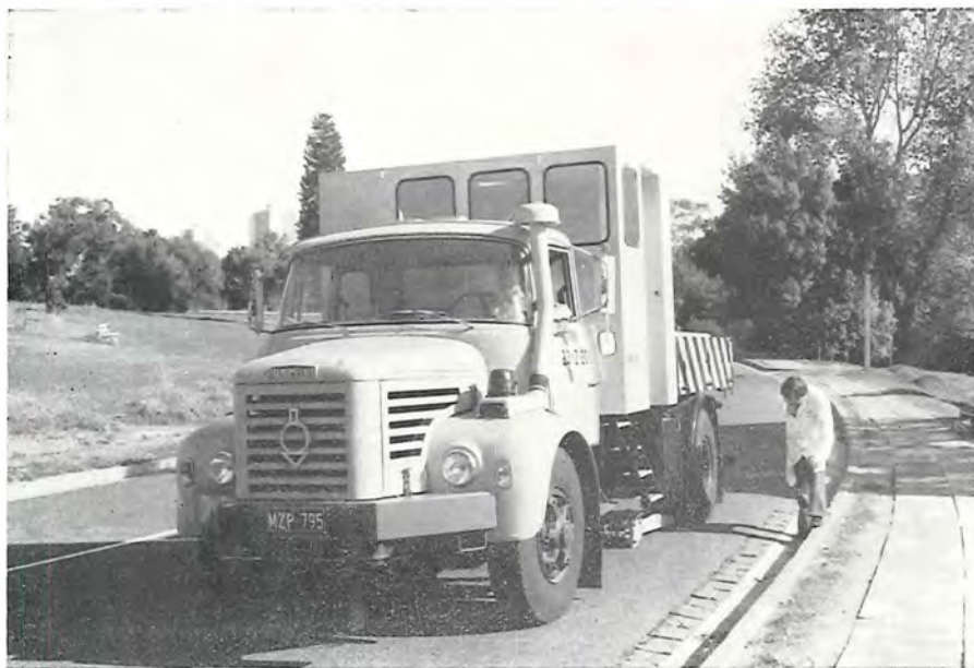
Plate 12—The Deflectograph in the testing mode.
