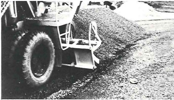
Plate 22: Aggregate loader showing the spiral and mouldboard extension.
