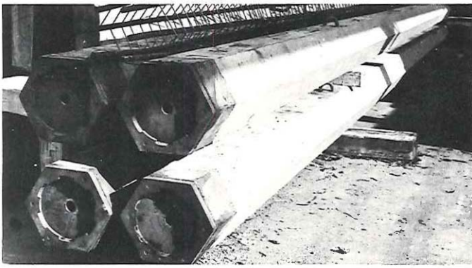
Plate 5 (above): Completed pile sections with female couplings.
