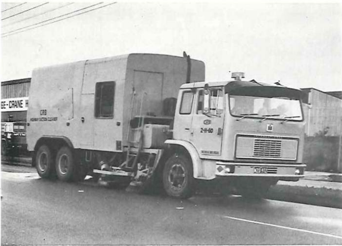
Plate 5: Highway suction sweeper
