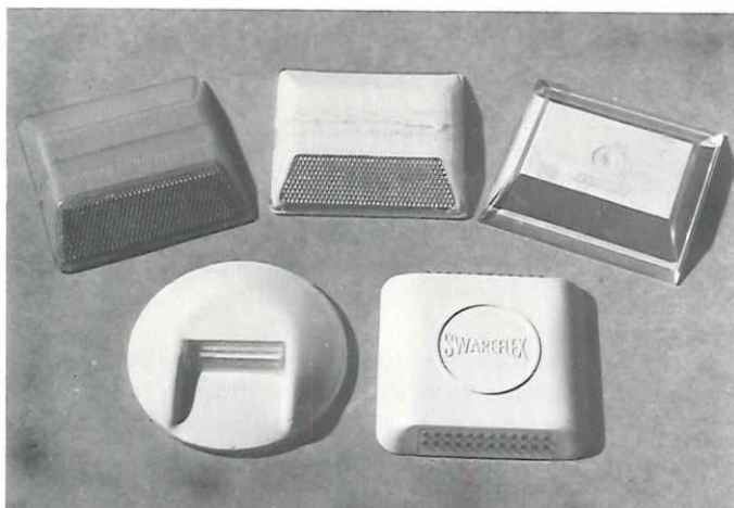
Plate 3: Raised reflective pavement markers (RRPMs) used in the Maroondah Highway service test: Upper row — Makes 1, 2 and 3; Lower row — Makes 4 and 5.
