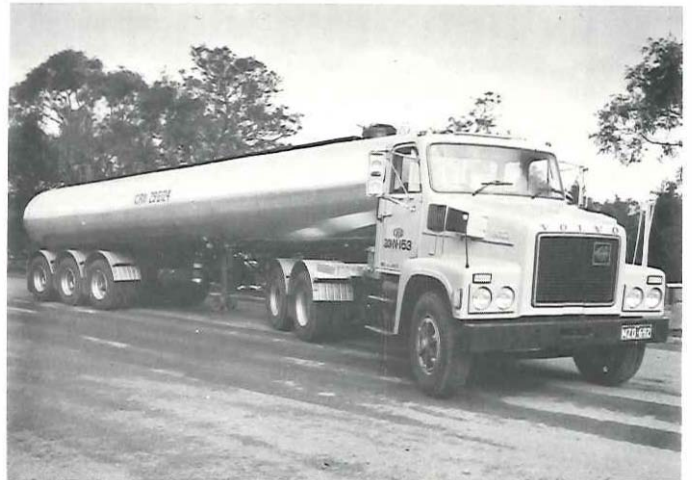
Plate 6: New 20,000 litre capacity bitumen road tanker
