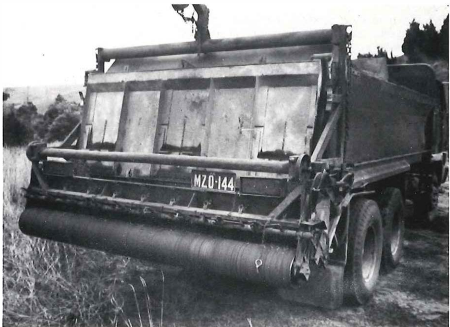
Plate 8: Truck mounted aggregate spreader
