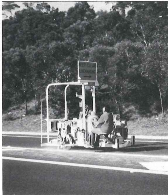
Figure 22: The Board's improved three-wheeled self-propelled roadmarker.
