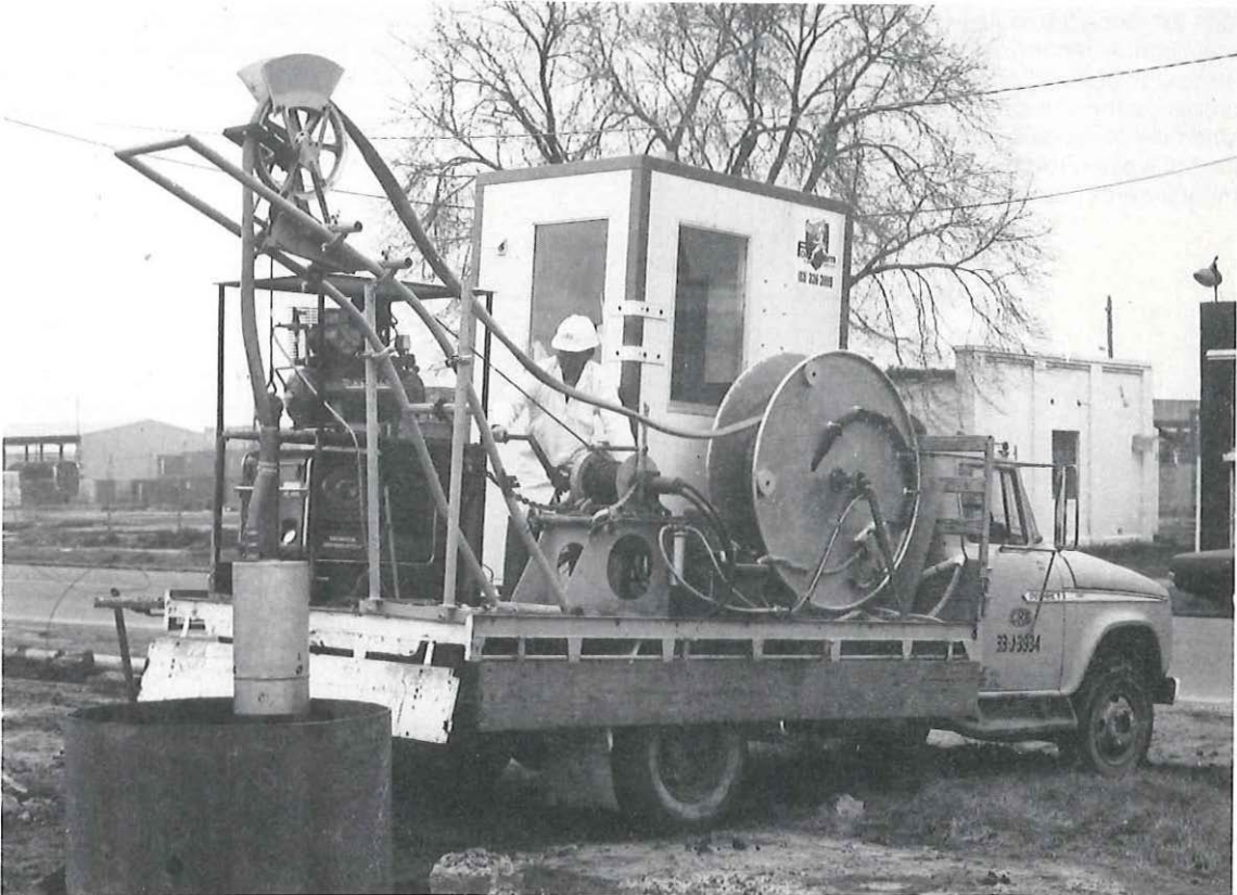
Figure 18. The Socket Inspection Device in operation.
