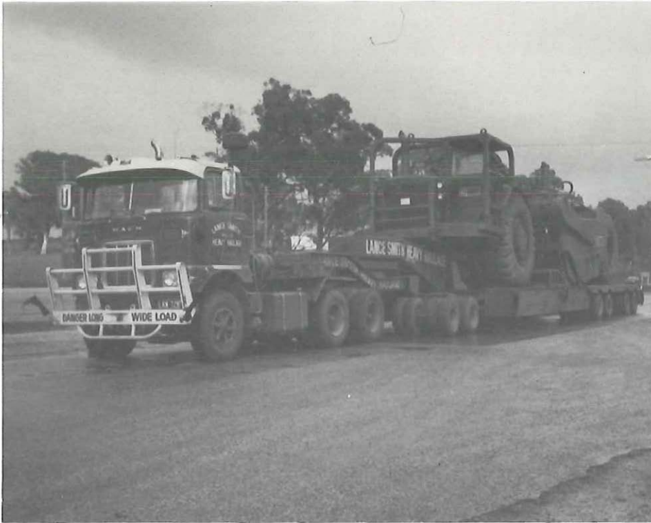
Figure 16 A 4.3 m wide low loader and CAT 641 Scraper at the Seymour weighbridge
