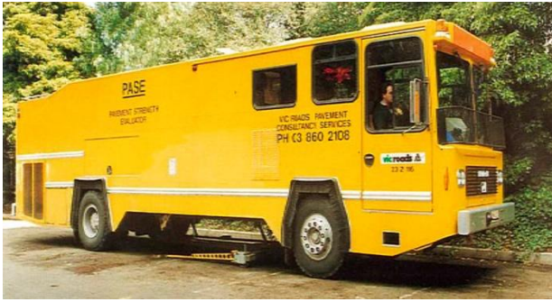
Pavement Strength Evaluator (PaSE) Cone Penetrometer Testing Vehicle
