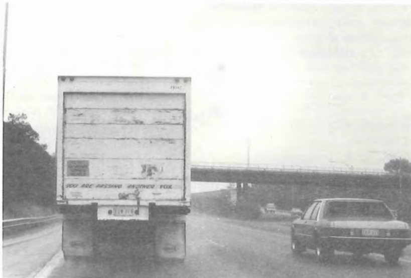
Figure 2. Same vehicle and conditions as Figure 1. Sprayed seal surface.
