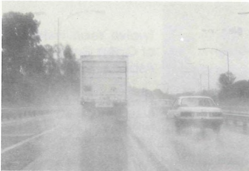
Figure 1. Water spray from heavy vehicle during steady rain. Dense asphalt surface.
