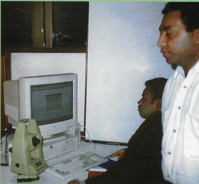
Downloading information from the Total Station (the device left of the computer monitor).
