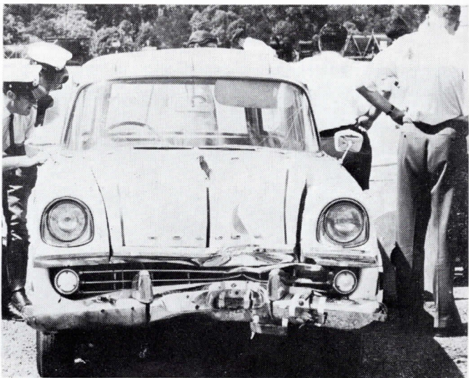
This test car collided with the light pole snapping it off at the base. Damage to the car was minor and restricted to outside bodywork.
