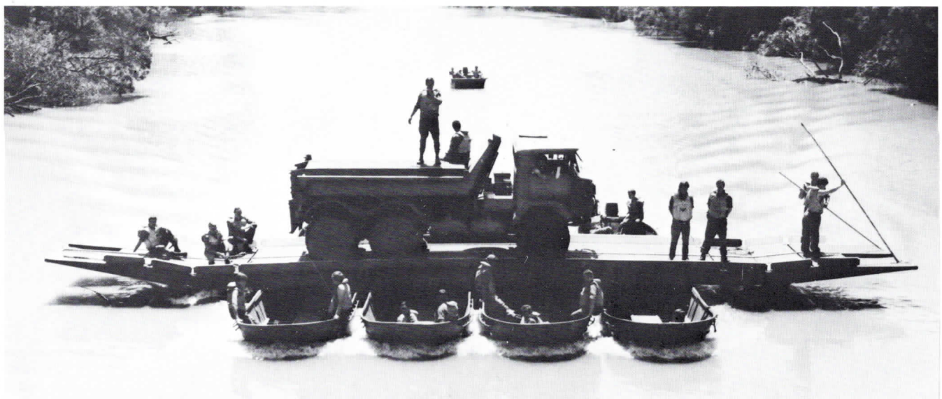
● Members of the regiment operate a light tactical raft on the Georges River.
