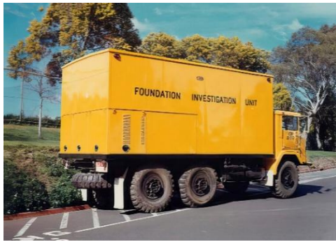
Cone Penetrometer Testing Vehicle
