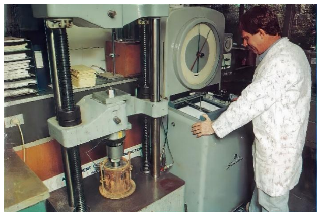
Vish MacKowski operating a modern CBR Testing Machine
