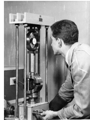
Anthony Rees conducting a Marshall Stability test
