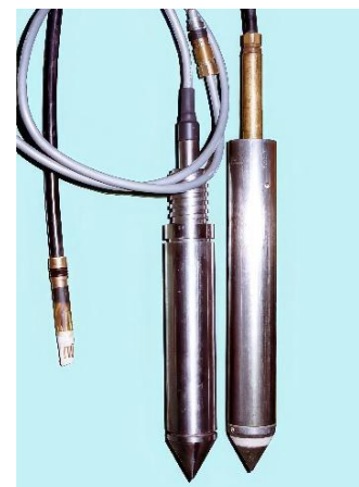
Piezo-Cone Penetrometer (R) and Friction Cone Penetrometer (L)
