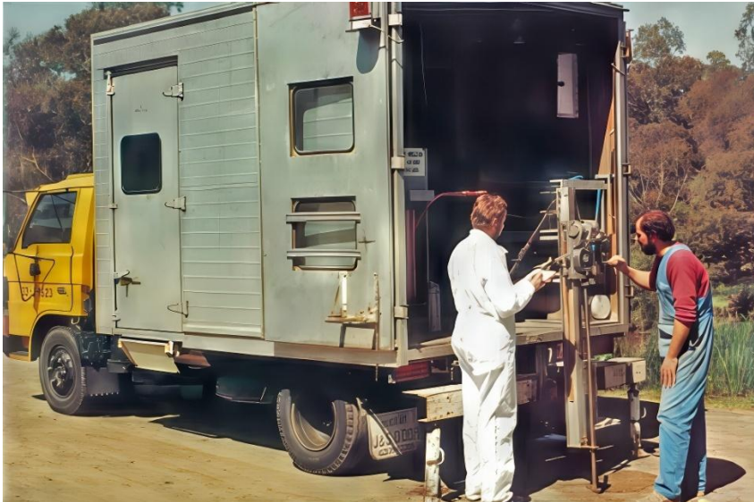
Static Cone Penetrometer – David Simpson, the operator (in white)
