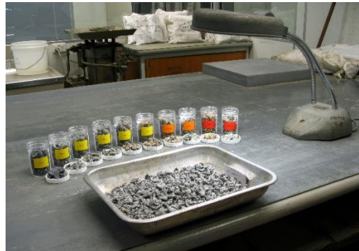
Assessment of Unsound Stone – Sample Jars of Sound, Marginal and Unsound Rock
