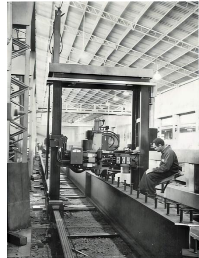
Production Friction welding machine
