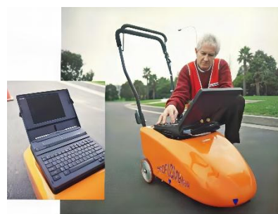
Photo of Ian Rogers with Hand Pushed Smoothness Measuring Device
