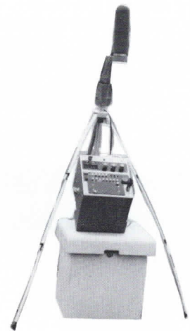
● A Community Noise Analyser . . . the CRB uses this equipment to record traffic noise.
